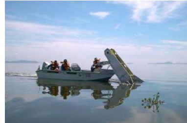
Fig. 32: Lamor Bow Collector 2 C2700
