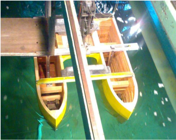
Fig. 16: Large Catamaran model in the towing tank
